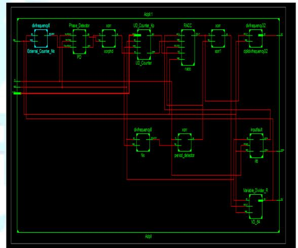
Fig 7: The RTL schematic view of ADPLL
