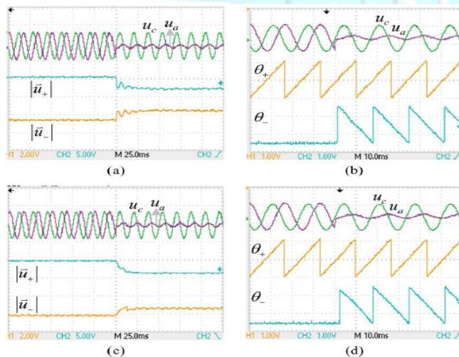
Fig 3: Positive and negative sequence detection during a single-phase fault
