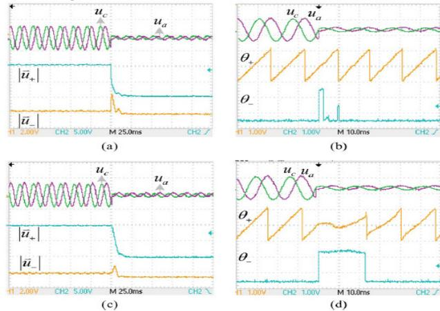
Fig 5: positive and negative sequence detection during a three-phase fault a) Voltage detected with ADPLL b) Phase angle detected with ADPLL.c) Voltage detected with SOGI PLL d) Phase angle detected with SOGI PLL
