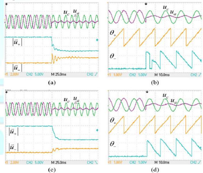
Fig 4: Positive and negative sequence detection during a two-phase fault a) Voltage detected with ADPLL b) Phase angle detected with ADPLL c) Voltage detected with SOGI PLL d) Phase angle detected with SOGI PLL
