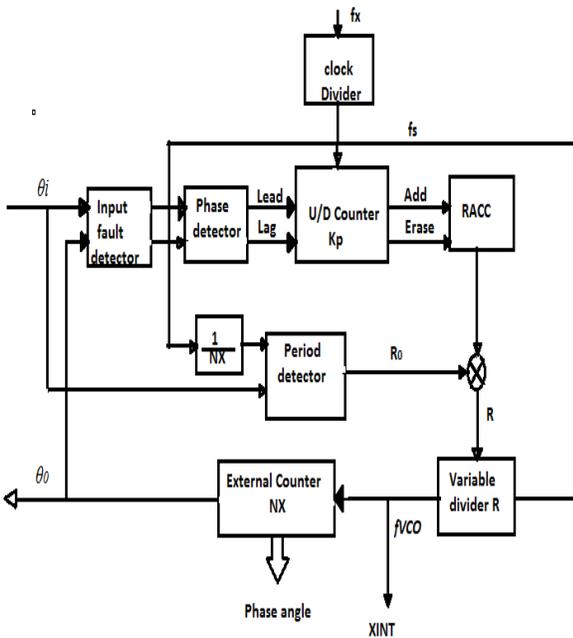
Fig.1, Block diagram of proposed ADPLL
